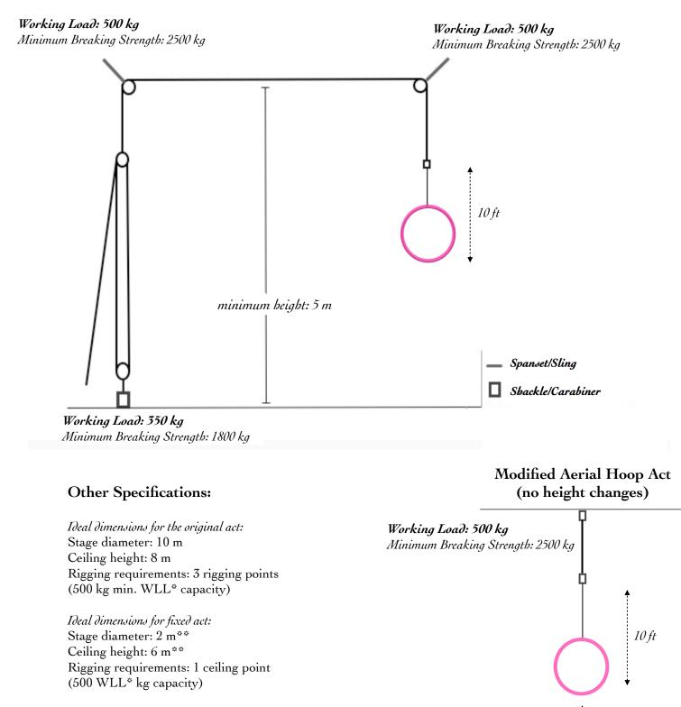
\*WLL = Working Load Limit \*\*Act can be adapted to fit alternatively sized spaces.
